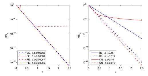
(a) Comparison of backward Euler (BE) and forward (b) Comparison of backward Euler (BE) and Crank-Euler (FE) scheme. Nicolson (CN) scheme.
