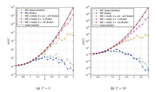
Figure 1: Monte Carlo simulations for the geometric Brownian motion (3) for  $\lambda = -1$ , and varying  $\sigma$ . All Monte Carlo simulations use  $M = 10^7$  trajectories.
