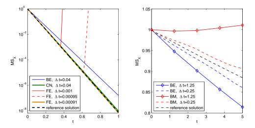
(a) Comparison of backward Euler (BE), Crank- (b) Comparison of backward Euler-Maruyama (BE) Nicolson (CN) and forward Euler (FE) schemes. and backward Euler-Milstein (BM) scheme.
